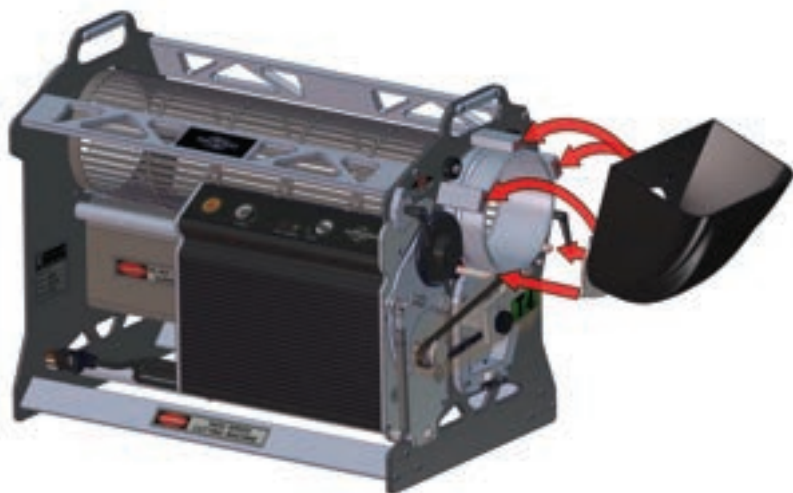
Figure 9: Installing the hopper
