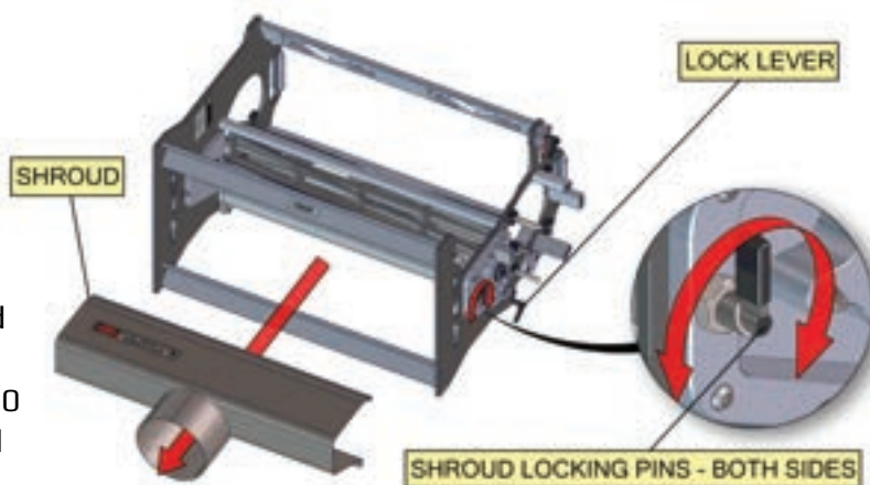
Figure 28: Removing the shroud
