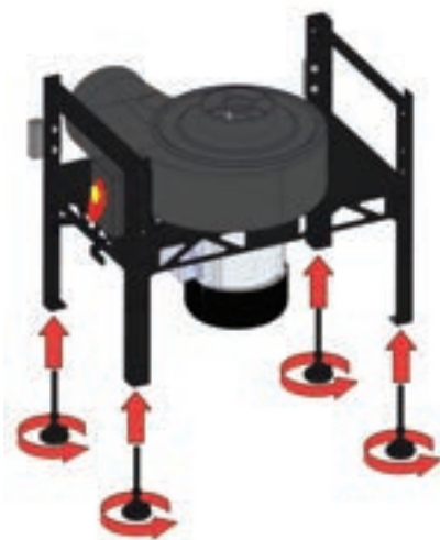
Figure 10: Installing feet on the leaf collector
