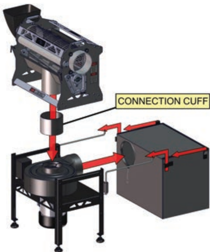
Figure 11: Connecting the T4 to the leaf collector
