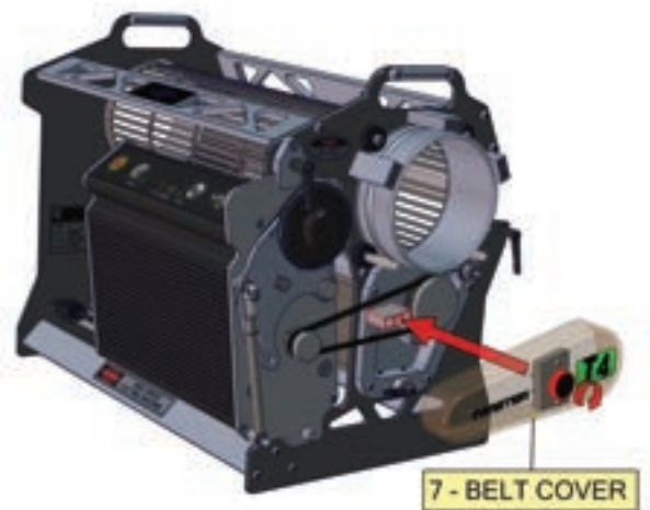
Figure 4: Installing the belt cover
