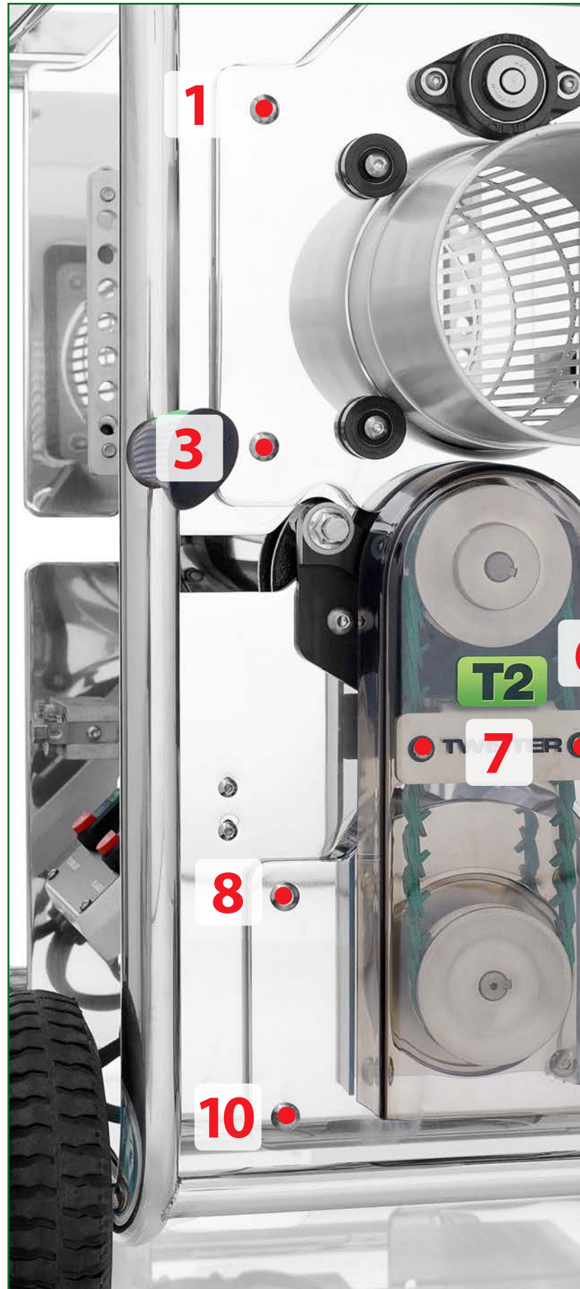
Figure 2.3 Tumbler adjustment and belt replacement
